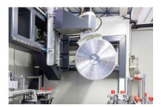
550 mm diameter saw that can cut at any angle between  $0^{\circ}$  and  $180^{\circ}$  thanks to its 4-axis movement capability, the saw allows cutting and end-milling operations of profiles up to 320 mm wide.
