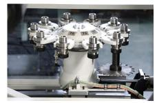
Thanks to its built-in automatic magazine with capacity for 8 tools, GARNET XS4 saves time when switching to different operations.
