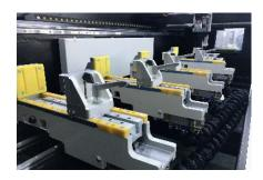
With full automatic clamp positioning, GARNET XS4 automates many tasks assuming the work load of the user.
